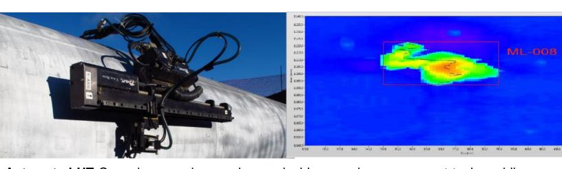
**Automated UT** Corrosion mapping can be a valuable corrosion assessment tool providing an image (C-Scan) of the affected area in conjunction with Burst Pressure Calculations (B31.G, MB31G and Effective Area Assessment).
