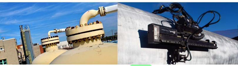
Automated UT Corrosion mapping can be a valuable corrosion assessment tool providing an image (C-Scan) of the affected area in conjunction with Burst Pressure Calculations (B31.G, MB31G and Effective Area Assessment).
